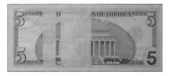
true advantages of IR printing is its capacity to be rendered into "machine readable" characters or features that allow for automated validation by a machine, such as a bill acceptor on a vending machine, or a high-speed money counting machine. The image above shows the appearance of a US \$5 bill under infrared light. The two "bars" are precisely located and can be easily "seen" and "read" by machines.
