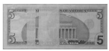
Referring again to this image of the \$5 US banknote under IR light, the two "bands" seen here can be used as a basis for identification by an intelligent device, programmed with data regarding the location(s) & width(s) of this feature. Similarly, the IR features of the other
