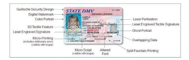
Pictured here is a rendering, provided to us by L1 Identity Technologies, Inc. which shows the number and diversity of different security design elements that may be included in a single secure document design. This is not a comprehensive listing of such features, but rather, is an illustration that one document may contain dozens of individual design features that can be used in a pattern-matching application.
