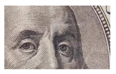
Because it is so difficult to reproduce both the resolution and the physical characteristics of intaglio printing, it is our opinion that, of all the "overt" features that can be used to verify documents – looking to authenticate the intaglio printing is the first-choice technique. This, of course, assumes that the document has intaglio printing.
